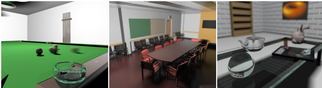
Figure 2.3: Examples of visual effects generated using distributed ray tracing, from left to right motion blur, soft shadows, and depth of field. Images from [Boulos et al., 2007].
